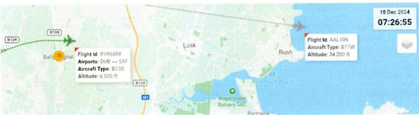
In the case of these two flights, the noise difference is 12dB (58dB for the South Runway flight & 70dB for the North Runway flight). While the level of noise varies from flight to flight, the general principle
